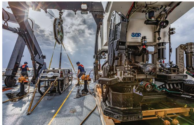
The team preparing the ROVs for deployment. During the **Deep Connections 2019** expedition, NOAA ROV *Deep Discoverer* will be used to acquire high-definition visual data and collect limited samples in poorly explored deepwater areas.
