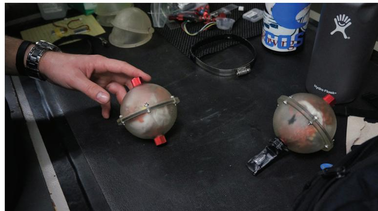
These pressure chambers were printed at sea by the URI team using their 3D printer. They were sent to a depth of 200 meters (656 feet) and successfully recovered intact, without any leaks or structure failures. To the team's knowledge, this is the first documented time this type of device has been printed at sea and then tested at depth. *Image courtesy of the NOAA Office of Ocean Exploration and Research, Mapping Deepwater Areas in the Caribbean and South Atlantic Bight.*
