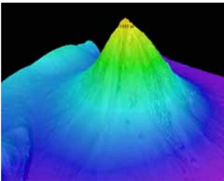
This is a perspective view of the Kawio Barat (West Kawio) seamount looking from the north-west acquired with multibeam sonar. The underwater volcano rises around 3800 meters from the seafloor. Image courtesy of NOAA *Okeanos Explorer* Program, INDEX-SATAL 2010. [http://oceanexplorer.noaa.gov/okeanos/explorations/10index/logs/hires/june26fig1\\_hires.jpg](http://oceanexplorer.noaa.gov/okeanos/explorations/10index/logs/hires/june26fig1_hires.jpg)
