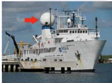
All communications with the shore are made possible by the *Okeanos Explorer*'s powerful satellite dome, which enables the ship to establish high-bandwidth connectivity with Exploration Command Centers throughout the world. Image courtesy of NOAA *Okeanos Explorer* Program, INDEX-SATAL 2010
