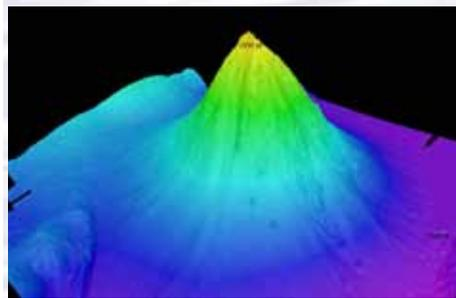
*Okeanos Explorer*'s EM302 multibeam sonar mapping system produced this detailed image of the Kawio Barat seamount, which rises around 3800 meters from the seafloor. Image courtesy of NOAA *Okeanos Explorer* Program, INDEX-SATAL 2010
