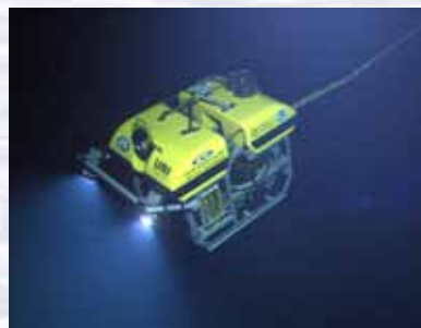
The ROV Little Hercules descends through deep water to an undersea volcano in the Celebes Sea to search for hydrothermal vents and associated ecosystems. Image courtesy of NOAA Okeanos Explorer Program, INDEX-SATAL 2010 http://oceanexplorer.noaa.gov/okeanos/explorations/10index/logs/hires/1june29_hires.jpg
