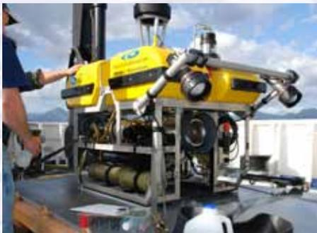
The *Little Hercules* remotely-operated vehicle (ROV) is a dual-body system capable of operating to depths of 4,000m. It is deployed from the *Okeanos Explorer* and attached to it by a tether. One vehicle is suspended above the other and serves to illuminate and image the surroundings. Image courtesy of NOAA Office of Ocean Exploration and Research.
