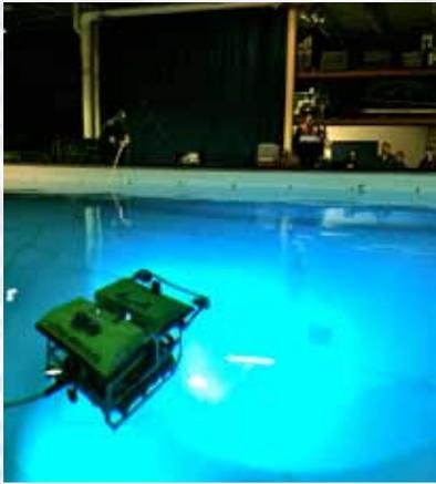
The *Little Hercules* ROV at the University of New Hampshire during tank testing. Image courtesy of NOAA *Okeanos Explorer* Program, INDEX-SATAL 2010.
