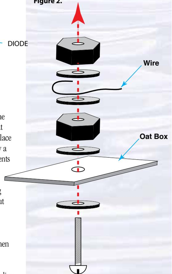
If you do not plan to use solder connections, place a flat washer on a machine screw, then push the screw through one of the holes from the inside of the oat box. Then place another washer onto the screw, and fasten the assembly in place with a 6-32 nut. Place two more washers onto the machine screw followed by a second nut. Do not tighten the second nut until all of the wires and components are in place (see Figure 2).
