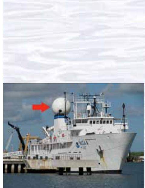
All communications with the shore are made possible by the *Okeanos Explorer*'s powerful satellite dome, which enables the ship to establish high-bandwidth connectivity with Exploration Command Centers throughout the world. Image courtesy of NOAA *Okeanos Explorer* Program, INDEX-SATAL 2010
