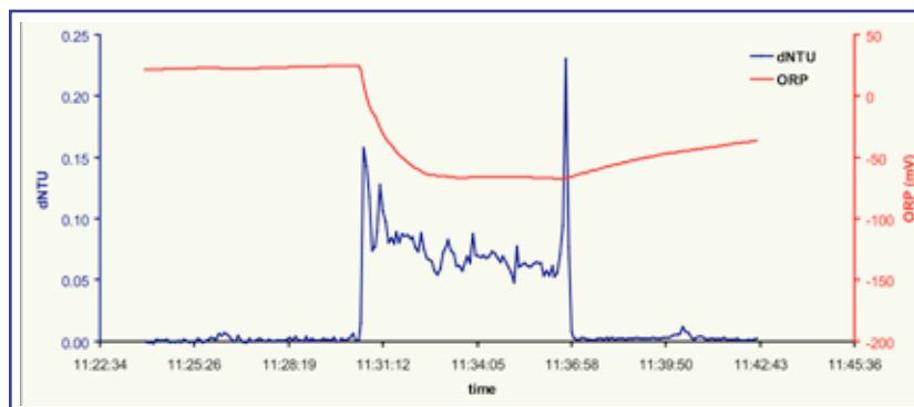
Plot showing light scattering (dNTU) sensor and oxygen reduction potential (ORP) data, versus time, acquired by the CTD/rosette as it passed through a plume overtop of Kawio Barat volcano. There was an intense particle anomaly and ORP decrease in the bottom 30 meters of the water column when the plume was encountered. A drop in the ORP, like you see here, means that there are more electron donor compounds in the water produced by enrichment of seawater in dissolved metals and chemicals billowing out of hydrothermal vents. The ORP values begin to increase again, recovering slowly, when the CTD leaves the plume. Image courtesy of Sharon Walker, PMEL.
