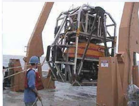
ROPOS being deployed for deepwater operations inside its steel cage.
