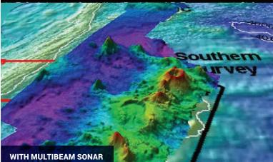
The top image shows what we previously knew about the seafloor terrain in the Southern Mariana region from satellite altimetry data. The bottom image includes an overlay of the information provided by *Okeanos Explorer*'s EM302 Multibeam System. *Image courtesy of NOAA OER.*
