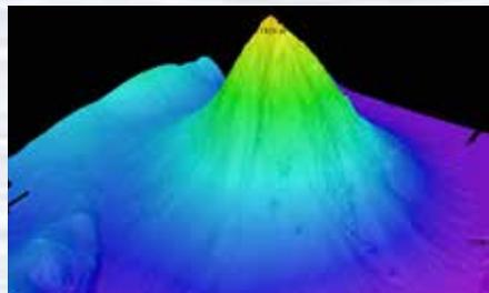
*Okeanos Explorer*'s EM302 multibeam sonar mapping system produced this detailed image of the Kawio Barat seamount, which rises around 3800 meters from the seafloor. Image courtesy of NOAA *Okeanos Explorer* Program, INDEX-SATAL 2010.
