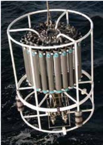
A CTD rosette with water sampling bottles attached is lowered to measure the salinity, temperature, depth and concentration of particles in the water column. Image courtesy of NOAA *Okeanos Explorer* Program, INDEX-SATAL 2010.
