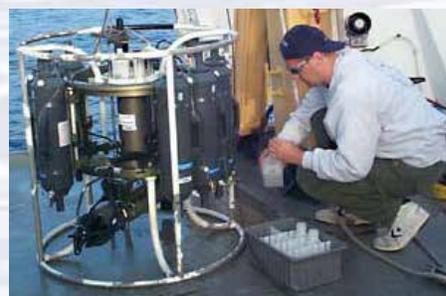
A CTD is attached to a metal frame called a rosette, or carousel, along with numerous water sampling bottles and when deployed, provides information about the composition of the water column. Image courtesy of NOAA. <http://oceanexplorer.noaa.gov/technology/tools/sondectd/sondectd.html>
