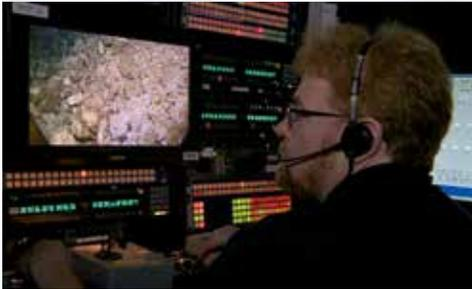
A video engineer adjusts the images from the HD camera on the remotely operated vehicle, *Little Hercules*. Image courtesy of the NOAA *Okeanos Explorer* Program.
