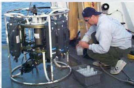
A CTD is attached to a metal frame called a rosette, or carousel, along with numerous water sampling bottles and when deployed, provides information about the composition of the water column. Image courtesy NOAA.
