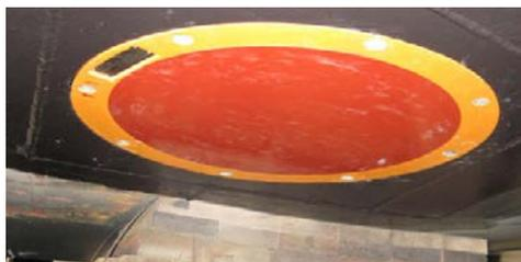
Picture of the EK60 split-beam transducer mounted on the hull of the *Okeanos Explorer*. Image courtesy NOAA Office of Ocean Exploration and Research. <http://oceanexplorer.noaa.gov/okeanos/explorations/ex1503/logs/jun6/media/ek60.html>
