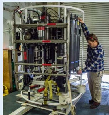
Water samples are collected from the Niskin bottles on a Conductivity, Temperature and Depth profiler (CTD). All 20 Niskin bottles take water samples from various depths, starting near the seafloor and ending close to the surface. Photo courtesy of Caitlin Bailey, GFOE, *The Hidden Ocean 2016: Chukchi Borderlands*. <http://oceanexplorer.noaa.gov/explorations/16arctic/logs/july24/media/shipton.html>
