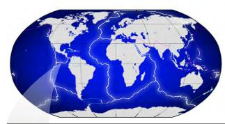
Length of MOR - 80,000km (2x circumference of Earth at the equator) nediate (>80mm/yr) Slow (>40mm/yr) Ultraslow (>20mm/yr) Length of MOR mapped at <100m resolution (<10,000km) Length of MOR mapped at <10m resolution (100km)
