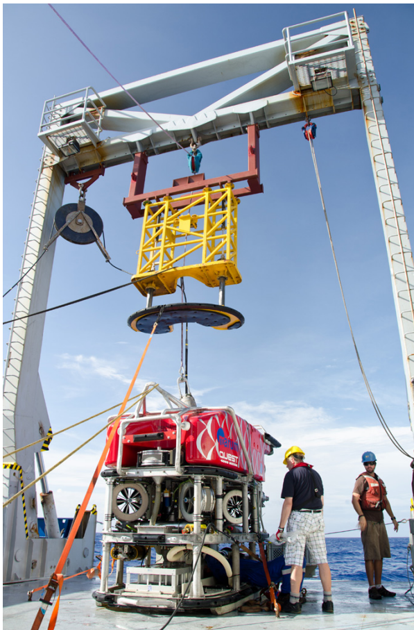
Fig 3.1-1. ROV QUEST on the main deck of RV Roger Revelle . The A-Frame is equipped with the umbilical block (left), main lift block (middle), the Launch and Recovery System (yellow) and custom built mounting adapters (brown parts). Image courtesy of Sean Diaz, SDProPho.
