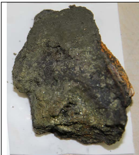
Fig. 6.1.2-7. Q328-sulfide-10 – Sample is approximately 8cm tall. Chimney sample dominated by chalcocopyrite.
