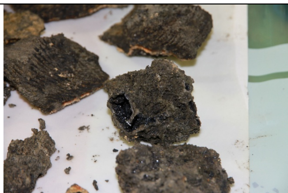
Fig. 6.1.2-3a. Sample Q323-sulfide-12. Sample pieces are approximately 4-5cm across. Entire sample is shown in photo 3b to the right.
