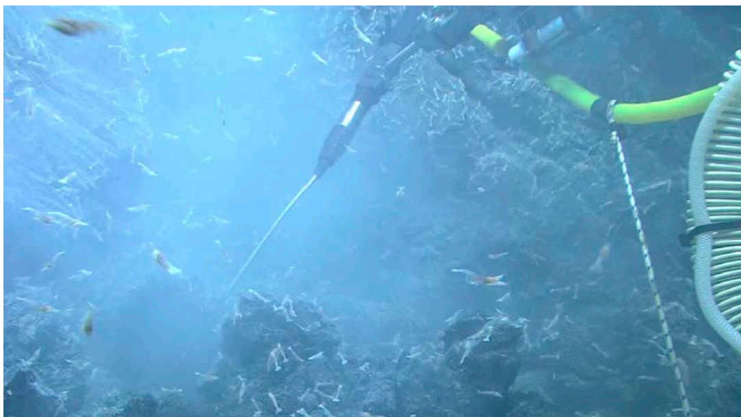
Fig. 3.1.1-1. Temperature probe in milky 10°C flow at Shrimp Plethora site during dive Q327 at West Mata.
