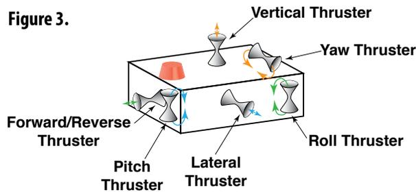
axis (but not at the middle of the axis) whose force is perpendicular to the axis, will cause rotational motion (Figure 3). If these thrusters are operated one at a time, though, they will also cause translational motion. To have only one rotational motion, two thrusters must be operated simultaneously so that the translational movements are cancelled out (Figure 4). The thruster arrangement shown in Figure 5 would be
