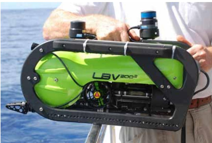
The SeaBotix LBV (little benthic vehicle) is a remotely operated vehicle (ROV) that researchers will use to explore potential underwater caves. Its small size (just 21 inches in length) makes it an ideal tool for exploring small underwater spaces. Image courtesy of Bermuda: Search for Deep Water Caves 2009 Exploration.
