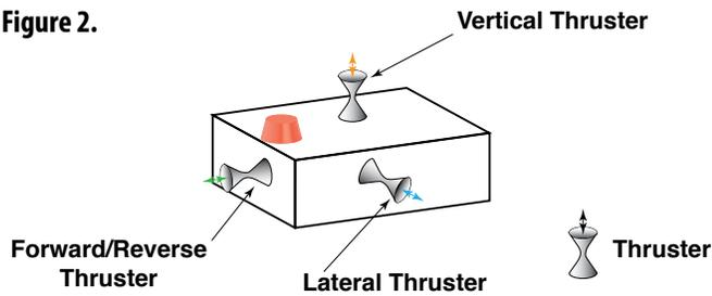
6. Have students complete Part B of the *Underwater Robot Motion Inquiry Guide*, then have each group present their results. If three thrusters are located so that the force of each thruster is directed exactly along a single axis, then these three thrusters will provide lateral, forward/reverse, and vertical motion along the x-, y-, and z-axes, respectively (Figure 2). Adding an additional thruster somewhere along each
