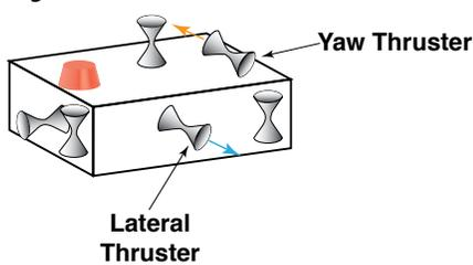
a better choice for an ROV that needed to have all six motions, since two thrusters could be operated in the same direction to obtain more power for translational motions, and could be operated with opposite rotations to spin the vehicle around a perpendicular axis.
