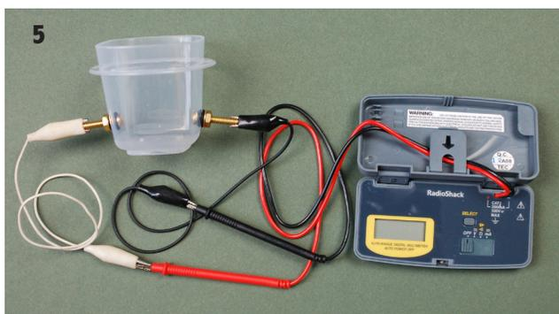
5. Attach one end of a jumper cable to one of the bolts, and the other end to one of the test leads on your ohm meter. Use a second jumper cable and repeat for the other bolt and other test lead. If you are using a multi meter, set the meter to measure resistance (ohms).
