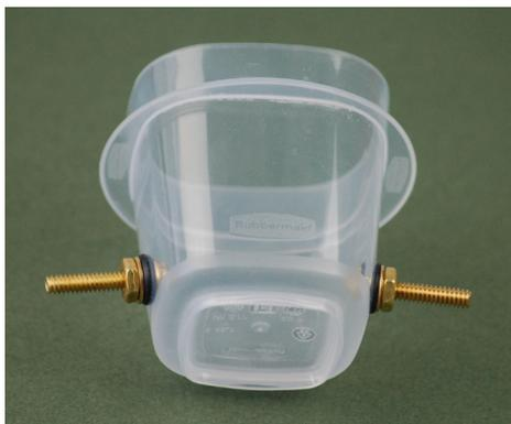
4. Pour water into the plastic container until it is about half full. Check to be sure no water is leaking around the bolt or grommet. If there is a leak, tighten the nut a little more. This assembly is called a conductivity cell.
