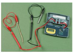
1. Start with two different metals. Set the voltmeter at its lowest setting, and connect the alligator clip on one end of a jumper cable to one of the probes from the voltmeter. Connect the alligator clip on the other end to one of the metals. Connect the alligator clip on one end of the other jumper cable to the remaining probe from the voltmeter, and connect the alligator clip on the other end to the other metal.
