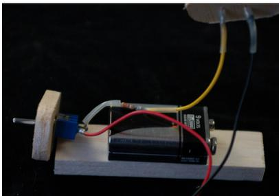
13. Bend the long lead of the resistor as shown so that it will fit over the battery, then glue the short pieces of wood to the ends of the long piece of wood using hot glue.
