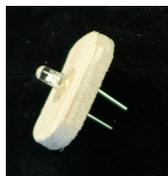
4. Bend the wire leads of the LED as shown so that the leads will fit through the 1/16" holes in the other short piece of wood. Put a small dab of hot glue on the wood between the holes, and hold the LED in place until the glue sets.
