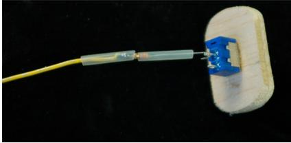
9. Put a 3/4" piece of heatshrink tubing over the other lead of the resistor. Bend the end of the lead into a U-shaped hook, and slide the hook through one terminal of the toggle switch. Crimp the hook tightly onto the switch terminal, then solder the connection.
