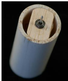
14. Check to be sure the switch is in the "Off" position (see Step 3). Attach the snap connector to the battery, and slide the assembly into the PVC pipe so that the piece of wood with the switch is flush with one end of the pipe. If necessary, use a small amount of hot glue to hold the assembly inside the pipe. Your Ultraviolet Illuminator is finished! Test your illuminator by turning the switch on in a darkened room. Remember: NEVER LOOK DIRECTLY AT A SOURCE OF ULTRAVIOLET LIGHT!
