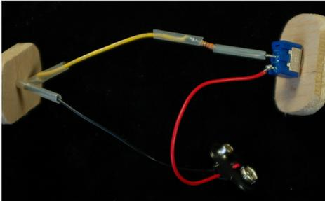
10. Remove about 1/4" of insulation from the red lead of the 9-volt battery snap connector, and twist the strands together. Bend the end of the lead into a U-shaped hook, and slide the hook through the other terminal of the toggle switch. Crimp the hook tightly onto the switch terminal, then solder the connection.
