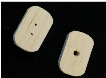
2. Drill two 1/16" diameter holes in one of the short wood pieces in the locations indicated on Pattern 1. Drill one 1/4" hole in the other short wood piece as indicated on the pattern.
