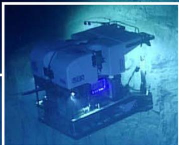
NOAA Ocean Exploration's remotely operated vehicle (ROV) Deep Discoverer surveys the Currituck submarine landslide off the eastern coast of the US. Technology like this makes the deep sea accessible to scientists, allowing for the study of this remote but critically important environment.
