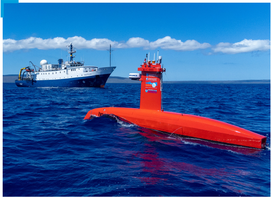
Numerous navigation and communication systems mounted on top of USV DriX allow it to operate autonomously or remotely-controlled from a pilot on land or on shore. Image courtesy of Ocean Exploration Trust.
