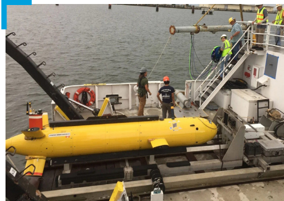
The large-bodied AUV Eagle Ray sits on top of its Launch and Recovery System (LARS), a unique ramp used to deploy it from the back of a research vessel like NOAA Ship Okeanos Explorer . Image courtesy of Leonardo Macelloni, University of Southern Mississippi.
