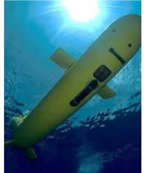
AUV Eagle Ray 's torpedo shaped body makes it very hydrodynamic, helping the vehicle to conserve power and map the seafloor for up to 30 hours per dive. Image courtesy of University of Southern Mississippi.
