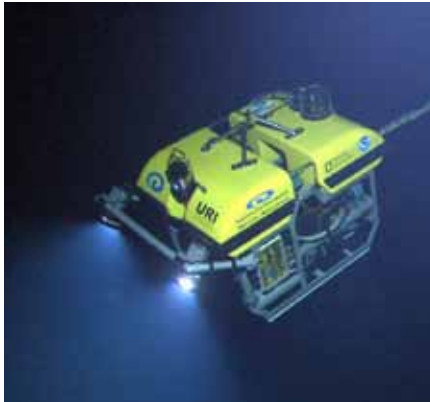
The ROV Little Hercules descends through deep water to an undersea volcano in the Celebes Sea to search for hydrothermal vents and associated ecosystems. Image courtesy of NOAA Okeanos Explorer Program, INDEX-SATAL 2010 http://oceanexplorer.noaa.gov/okeanos/explorations/10index/logs/hires/1june29_hires.jpg
