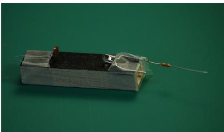
4. Tape the LED onto one end of the balsa wood.
