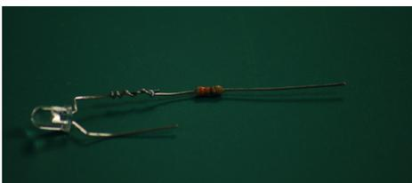
3. Notice that the base of the LED is flattened on one side. The lead that is closest to the flattened site is the cathode of the LED which connects to the negative side of the battery. Separate the leads of the LED as shown, and twist the 330 ohm resistor onto the lead that is NOT next to the flattened side (this is the anode of the LED).
