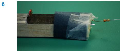
6. Tape one of the pieces of black construction paper over the LED so that it forms a dome. Press down on the end of the construction paper that is near the end of the balsa wood and tape it in place.
