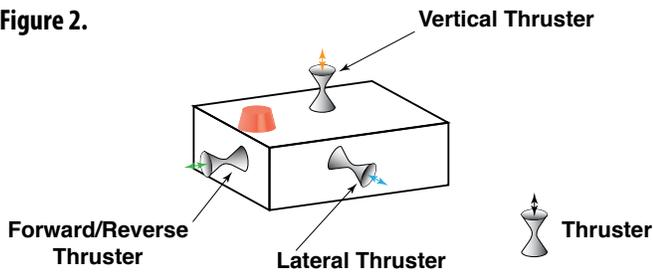
6. Have students complete Part B of the *Underwater Robot Motion Inquiry Guide*, then have each group present their results. If three thrusters are located so that the force of each thruster is directed exactly along a single axis, then these three thrusters will provide lateral, forward/reverse, and vertical motion along the x-, y-, and z-axes, respectively (Figure 2). Adding an additional thruster somewhere along each
