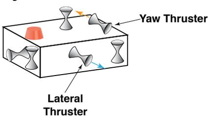
The thruster arrangement shown in Figure 5 would be a better choice for an ROV that needed to have all six motions, since two thrusters could be operated in the same direction to obtain more power for translational motions, and could be operated with opposite rotations to spin the vehicle around a perpendicular axis.
