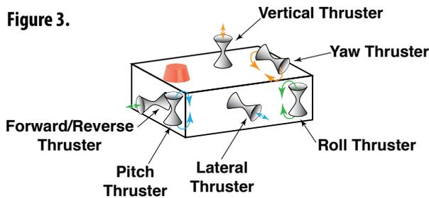
axis (but not at the middle of the axis) whose force is perpendicular to the axis, will cause rotational motion (Figure 3). If these thrusters are operated one at a time, though, they will also cause translational motion. To have only one rotational motion, two thrusters must be operated simultaneously so that the translational movements are cancelled out (Figure 4).
