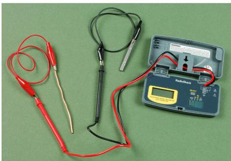
1. Start with two different metals. Set the voltmeter at its lowest setting, and connect the alligator clip on one end of a jumper cable to one of the probes from the voltmeter. Connect the alligator clip on the other end to one of the metals. Connect the alligator clip on one end of the other jumper cable to the remaining probe from the voltmeter, and connect the alligator clip on the other end to the other metal.
