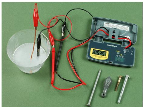
2. Pour about 100 ml of seawater into a plastic cup. Place the metals into the seawater so they are not touching, but are about 1 cm apart. Record the voltage reading on the voltmeter. If the needle on the voltmeter goes down or the reading is negative, reverse the probes.
