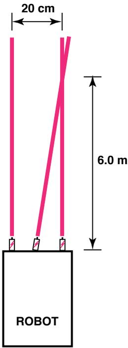
A similar system can be used in forward-looking video, but it is often important to be able to estimate distance as well. To provide this capability, a third laser is added to the system, in between the two parallel lasers. This additional laser is angled so that it converges with one of the parallel laser beams at a known distance in front of the robot (see Figure 2).
