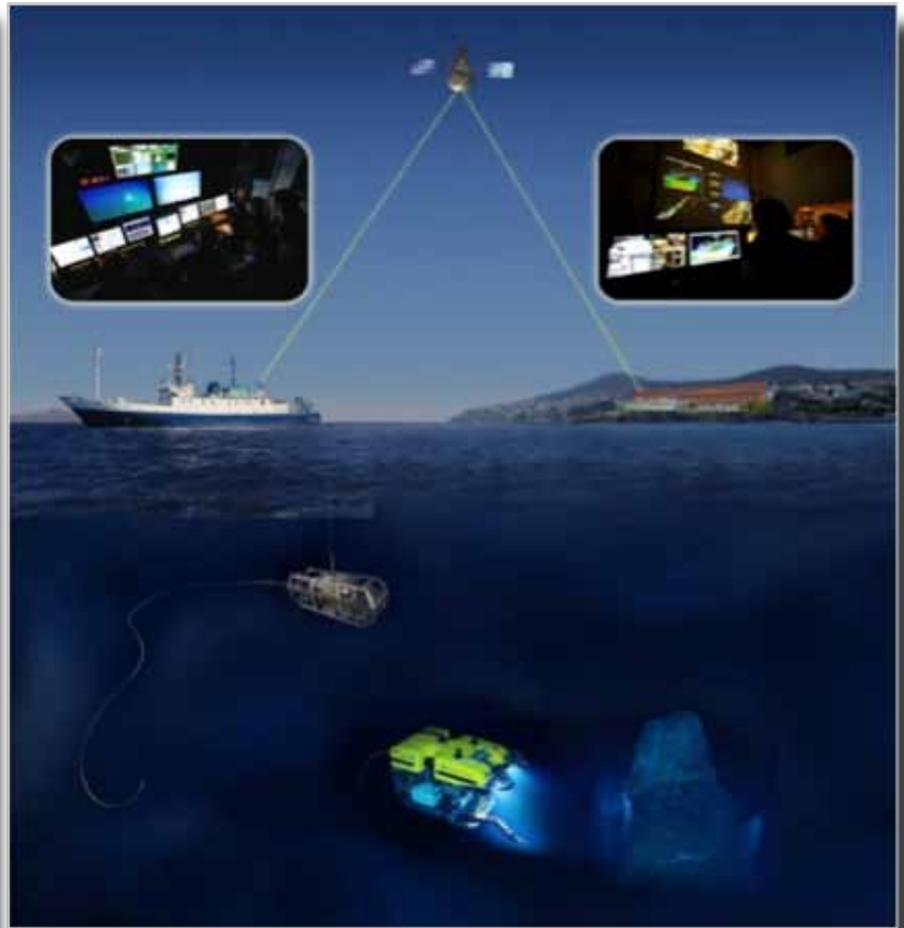
Diagram showing telepresence systems onboard a ship of exploration and the pathways connecting live video from undersea vehicles to the Inner Space Center and on to the internet. Credit: K. Cantner.
