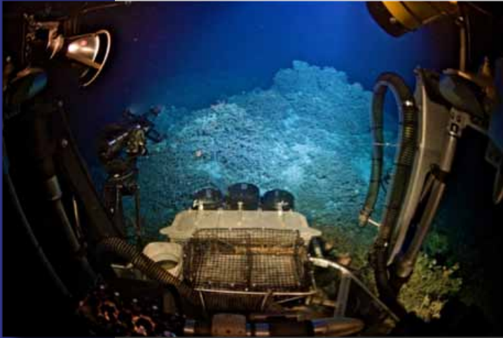
Inside the sphere of the Johnson Sea-Link submersible. Image courtesy of Art Howard, Life on the Edge Expedition , NOAA-OE.
