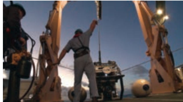
The author on stern of the NOAA Ship Okeanos Explorer overseeing deployment of the camera sled for a ROV dive.
