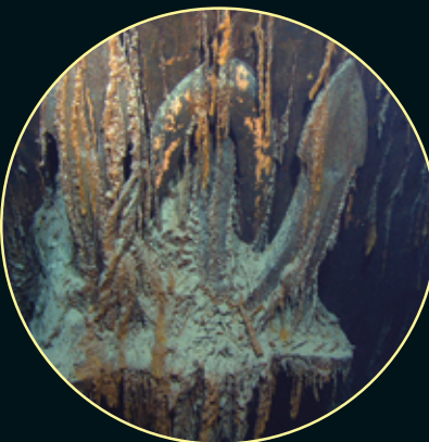
Rusticle formations on the hull and anchor. 2
