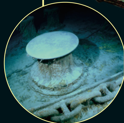
This large capstan used for handling lines is located on the starboard side of the forecastle deck. Memorial plaques can be seen on some capstans. These capstans serviced lines for the paired bitts along the rail. 1
