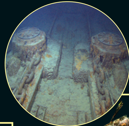
Windlasses and massive anchor chains on the forecastle deck. 2
