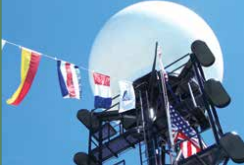
Okeanos Explorer's prominent VSAT (Very Small Aperture Terminal) dome enables satellite communications between explorers ashore and at sea and provides multiple high-definition video streams for widespread dissemination. Image credit: NOAA.
