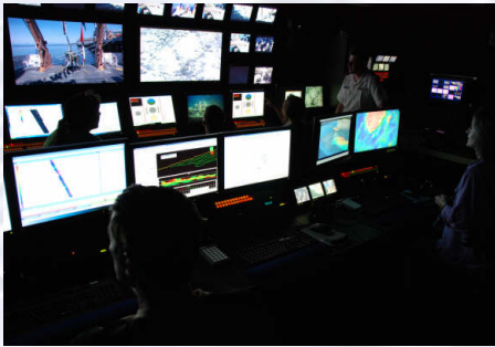
Okeanos Explorer's Control Room is the exploration heart of the ship, serving a number of missions including processing of multibeam sonar for mapping, controlling video transmitted off the ship, and coordinating the interaction between those afloat and ashore. When ROVs are deployed, they are controlled here by a navigator, pilot and co-pilot. Images from various cameras on the ship, and on deployed ROVs, can be brought up on the large screens. Image credit: NOAA.
