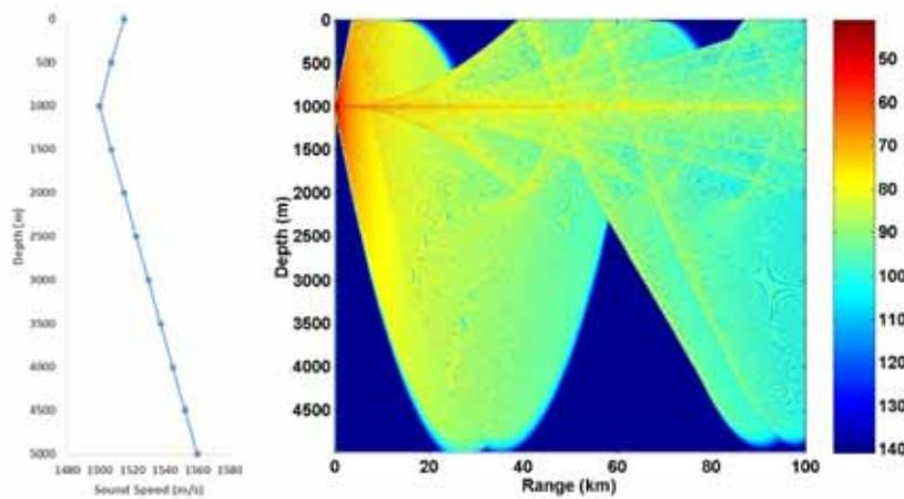
Figure 1. Propagation of a 200 Hz signal in the deep sound channel at mid-latitude with a source depth of 1000 m. Color bar = Transmission Loss (dB)
