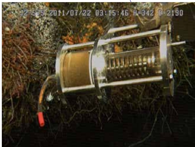
Syringe sampler used by ROV manipulators to collect microbial mat samples. Image courtesy of NOAA/NSF/WHOI.
