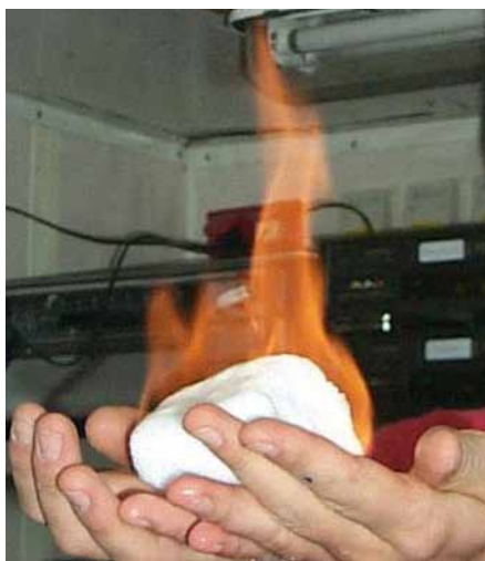
Methane hydrate looks like ice, but as the "ice" melts it releases methane gas which can be a fuel source. Image courtesy Gary Klinkhammer, OSU-COAS
