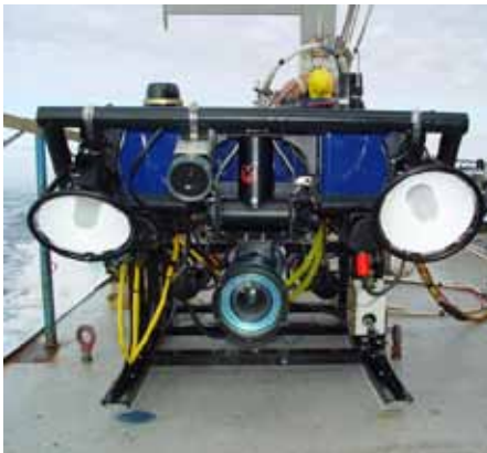
Helia, an ROV carrying a High Definition TV camera (foreground) and Isis, a towed sled with auxiliary lighting, sit on the stern of the RV Connecticut. http://oceanexplorer.noaa.gov/explorations/03portland/logs/sept15/media/helaisis.html
