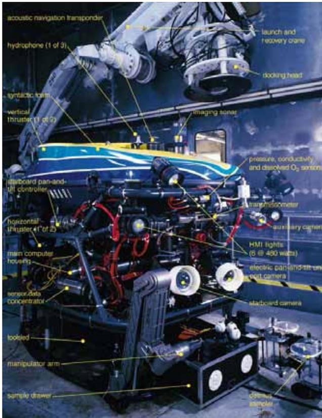
A detailed image of the sensors and sampling tools on the ROV Tiburon. Image courtesy of MBARI.
