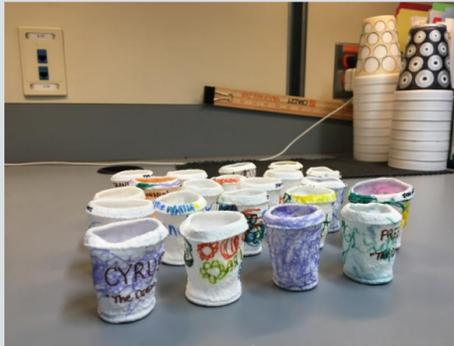
Styrofoam cups after visiting 2,500 meters deep attached to the ROV *Seirios*. Image courtesy of the NOAA Office of Ocean Exploration.
