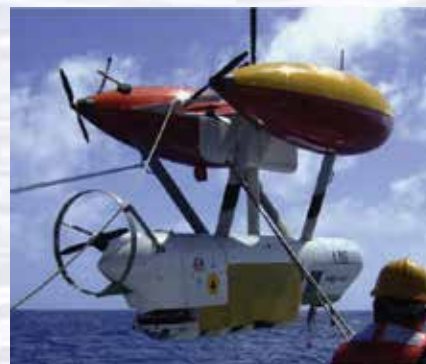
The ABE autonomous underwater vehicle (free-swimming robot). ABE (full name: Autonomous Benthic Explorer) has been used on multiple expeditions to find new hydrothermal vents in the deep ocean all over the world, from New Zealand to South Africa and from Brazil to Ecuador. Photo credit: Christopher German.
