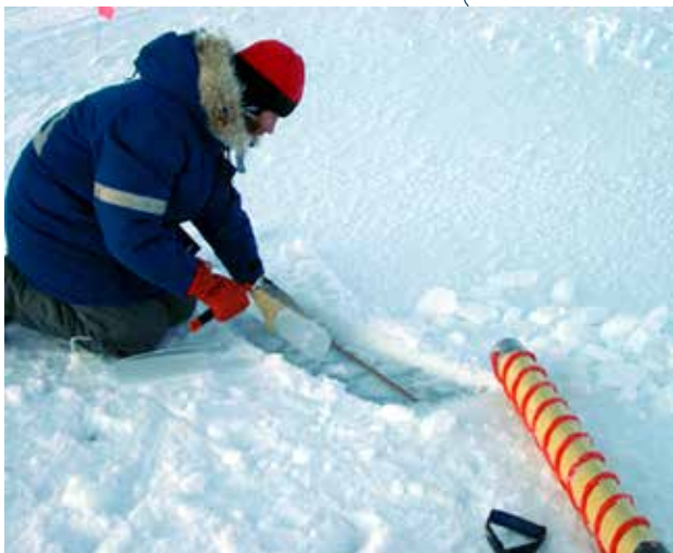
Sterilely sectioning a sea ice core in Franklin Bay, Canada. Image courtesy of Eric Collins.
