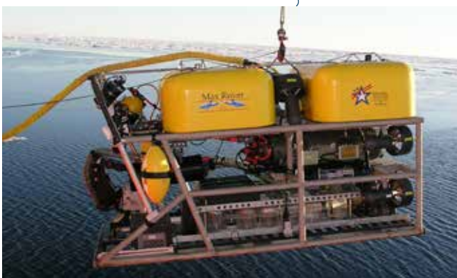
ROV Global Explorer will be used for both pelagic and benthic work. Equipped with new 4K cameras, this ROV will yield ultra-high-definition quality imaging of in situ habitats and communities, plus specimen collection capabilities essential for the discovery of delicate pelagic and benthic species. Image courtesy Deep Sea Systems.
