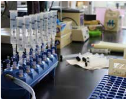
Vacuum pump apparatus for cleaning up and isolating genetic material. Image courtesy of the Mapping the Uncharted Diversity of Arctic Marine Microbes expedition.
